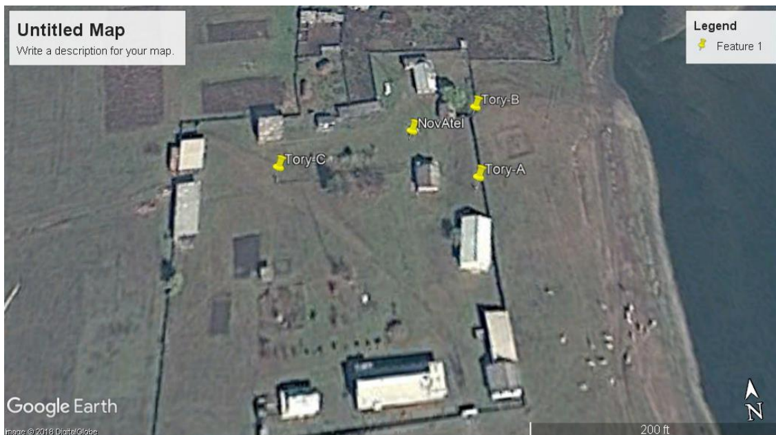
Figure 3. Location of receiving facilities in the Geophysical Observatory (Tory). Marks indicate locations of NovAtel receiver's antenna and three antennas of the JAVAD SigmaQ-G3T receiver (Tory-A, Tory-B, Tory-C)
