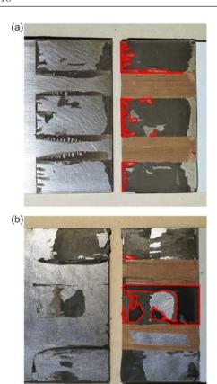
**Fig. 6.** Photographs of specimens of type #B after separation (kissing bonds marked with red lines): (a) #B.1; (b) #B.2.
