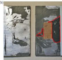
**Fig. 7.** Photographs of specimens of type #C after separation (kissing bonds marked with red lines): (a) #C.1; (b) #C.2.
