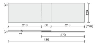
**Fig. 3.** The geometry of analysed adhesive joint: (a) plane view; (b) side view.
