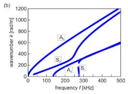
**Fig. 2.** Dispersion curves calculated by the transfer matrix method: (a) steel 3 mm plate; (b) two steel 3 mm plates joined with an adhesive with a thickness of 0.2 mm.
