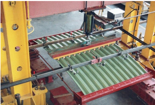
Fig. 4. Experimental setup with double arched sheet metal panel. The tie and deformation measurement method are visible. The load is applied at the arch crown (point C in Fig. 5a).
