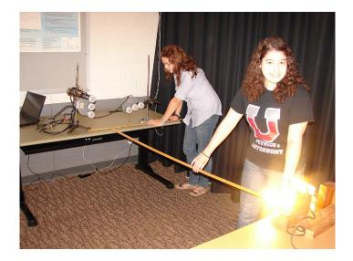
**Figure 2.** Union College students working with the VSRT. Two "triple" DirecTV feeds, taken from TV satellite dishes, used here as radio antennas, receive and detect the radio emission from compact fluorescent light bulbs (CFLs). Only one feed of each triple is active. The CFLs can be moved to assorted separation distances. The output spectrum from the interferometer is displayed on the laptop screen, and the data files are recorded.
