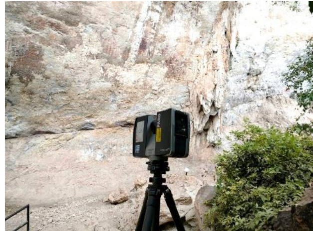
Figure 3: The Faro Focus 3D TLS used in the study.
