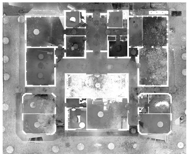
Figure 4. 3D laser scanner survey: the orthophotos of the facade, ceilings and floor plan.
