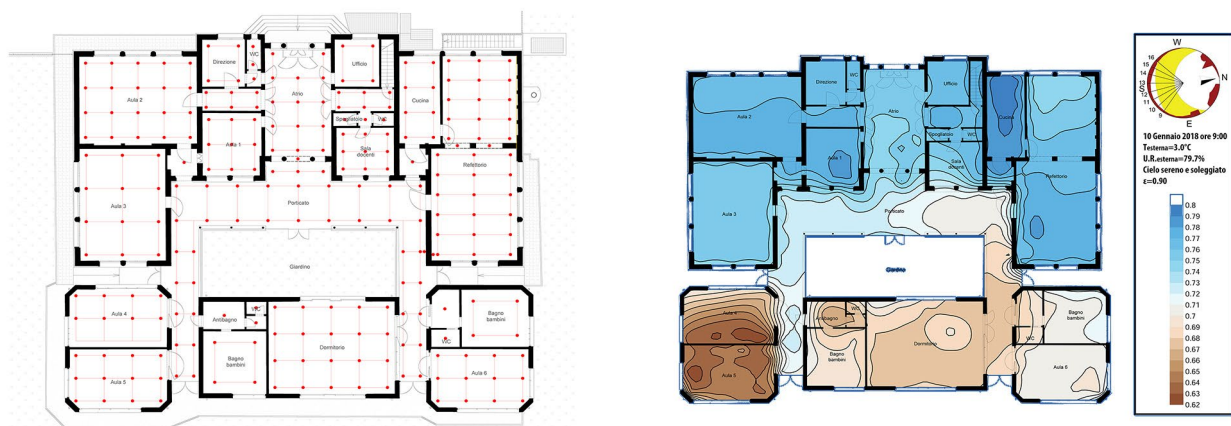
Figure 8. The mapping of the diagnostic analyses on the surface: thermo-hygrometric monitoring of the premises.
