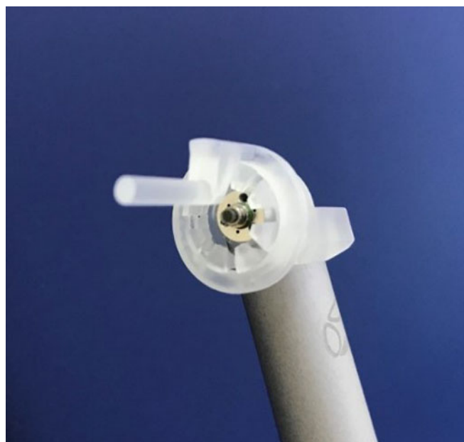
Fig. 2. Adjustable spacer, providing tip-to-tissue distance 10 mm, developed for the study.
