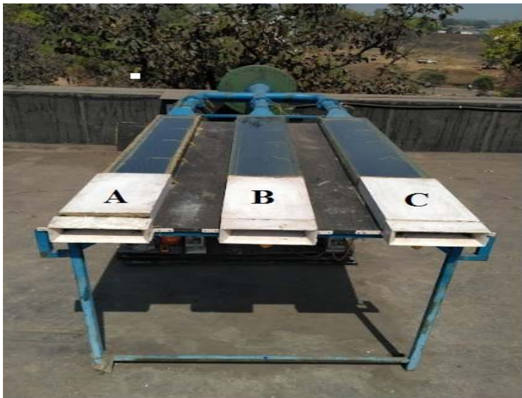
Figure (2): Photograph of the experimental set-up. (A) One side roughened duct; (B) Non-roughened duct; and (C) Three sides roughened duct.
