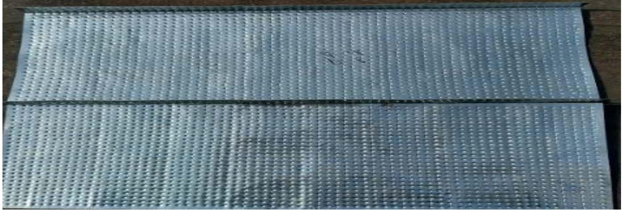
Figure (1): Typical one side and three sides concave dimple roughened
