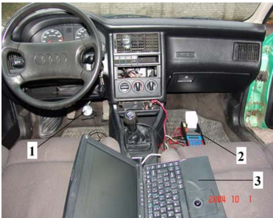
Fig. 2. Location of the experimental equipment inside the car: 1 – sensor of the brake pedal press strength; 2 – decelerometer VZM 100; 3 – the portable computer DELL LATITUDE XPi
