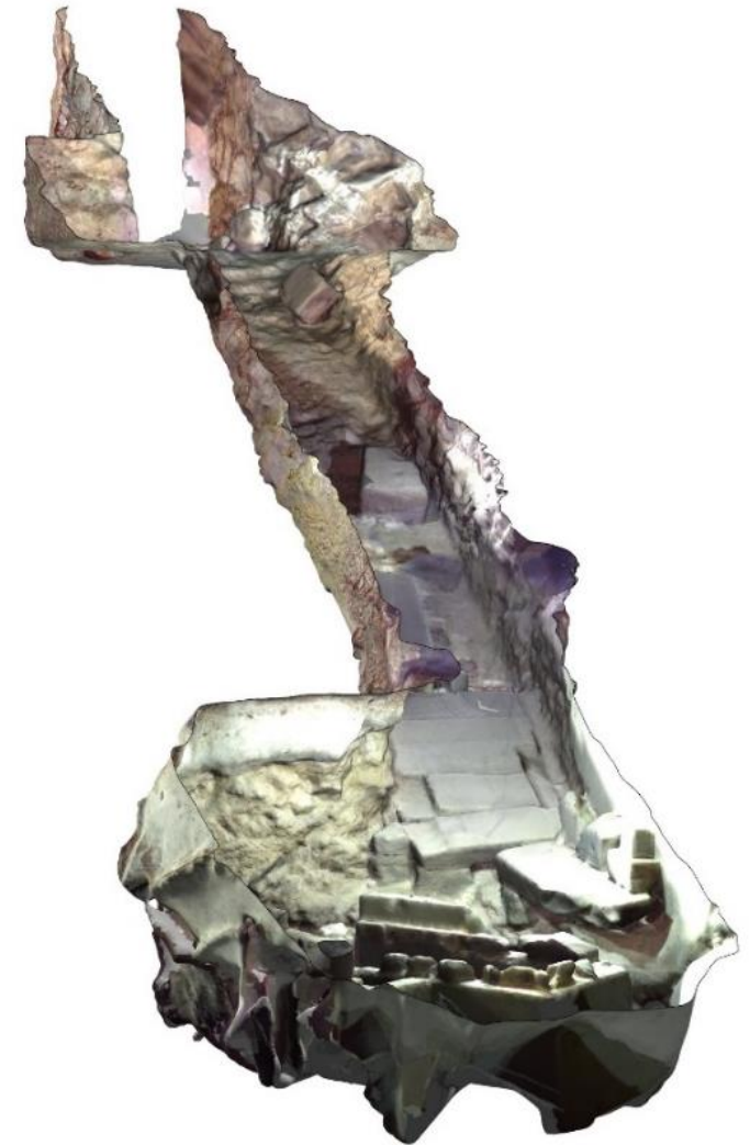
Figure 9: Post-processing mesh. Cleaning alternative through regenerating the geometry with a parametric algorithm, 2018
