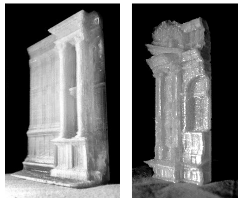
Figure 3: 3d printed fragments of the façade. FDM print in PETG plastic, 2017.
