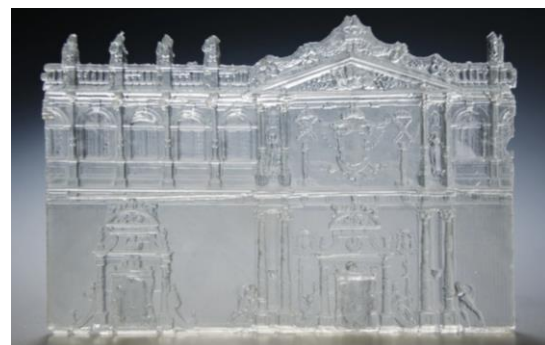
Figure 4: 3d printed fragment of the façade. SLA print with clear resin, 2017.
