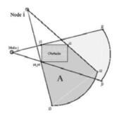
Fig. 3. Obstruction cones of nodes i and j around the obstacle [3]
