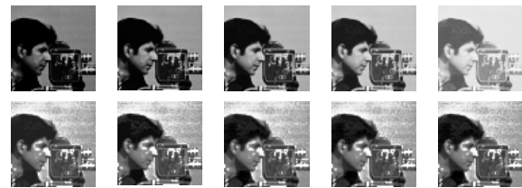
Figure1. The cameraman image with different brightness levels, in the first row, and the histogram equalized versions of each image, in the second row.
