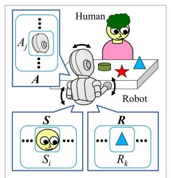
**FIGURE 1** Problem setting of the face-to-face interaction of the robot with a human caregiver. They sit across a table, and there are some objects on the table. The robot can produce actions such as moving head and hands as illustrated with the arrows in the figure. During the interaction with the human, the sensory data, taken actions, and resultant observations are stored in the sensory, action, and resultant variables, respectively (S, A, and R).
