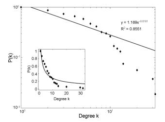
Figure 6. Cumulative degree distribution fitting power-law distribution is expressed in double logarithmic coordinate system. The inset figure is the cumulative degree distribution fitting power-law distribution in general coordinate system
