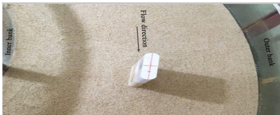
Figure 4. A view of the rectangular pier with an oblong nose, located in the 90 degree position in the 180 degree sharp bend
