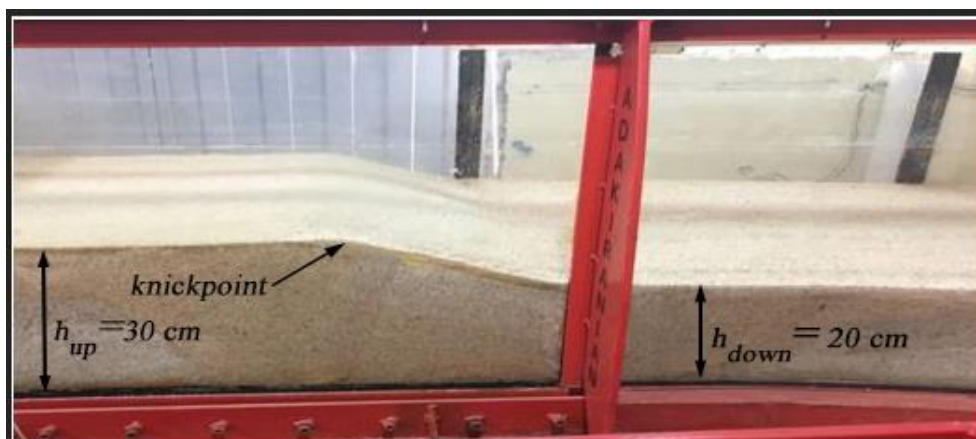
Figure 3. Base-level fall from the beginning of the bend to the end of the downstream straight path
