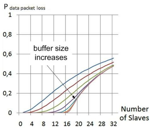
Fig. 4. d) Slave speed channel = 40 Mbps, Host speed channel = 400 (SpW max) Mbps, network load = 60%
