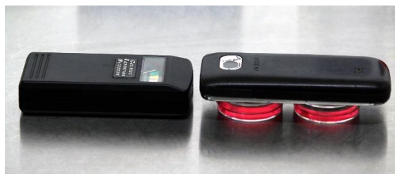
Figure 1. Set up for exposure of the cultured cells to mobile phone RFR
