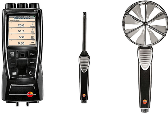
Fig. 3. The device which is used to measure air humidity, temperature and velocity
