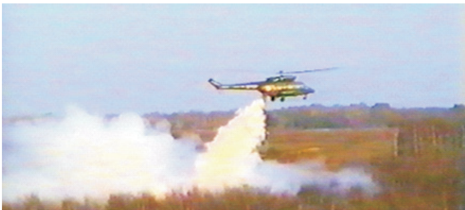
Fig. 35. PWD aboard a W-3WA helicopter: a spot smoke screen in deployment
