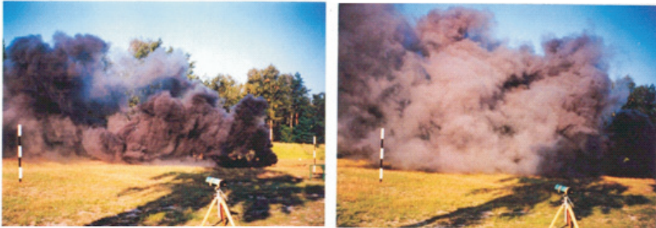
Fig. 15. Smoke screen shown in visible light as generated by a DM-2B small smoke candle. A laser transmission meter unit is shown in the foreground [14].
