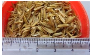
Fig. 2. Cleaned, washed and dried RH, which is in yellowish colour.
