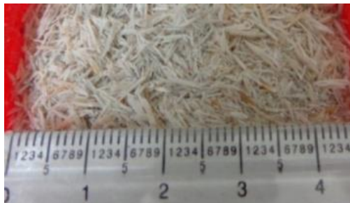
Fig. 4. White ash after thermal treatment.
