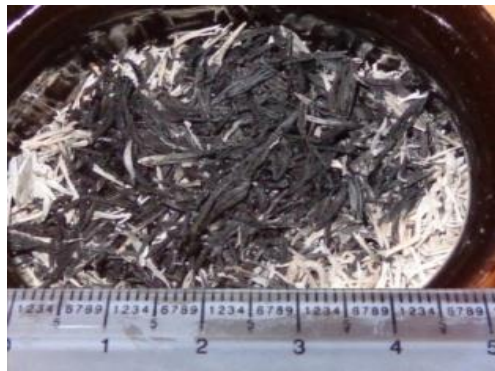
Fig. 3. Grey coloured incompletely combusted rice husk.
