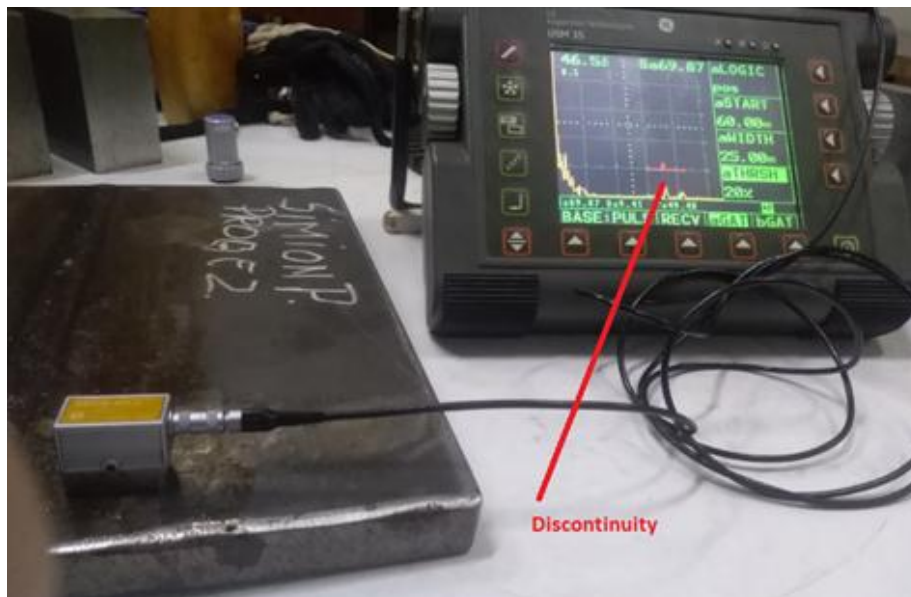
Figure 8 Detection of the discontinuity
