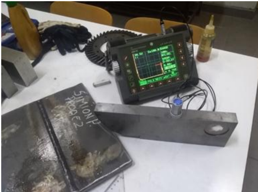
Figure 3 Calibrating the defectoscope with block A1
