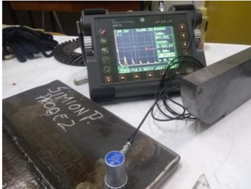
Figure 4 Ultrasonic examination with longitudinal waves on the left side of the joint
