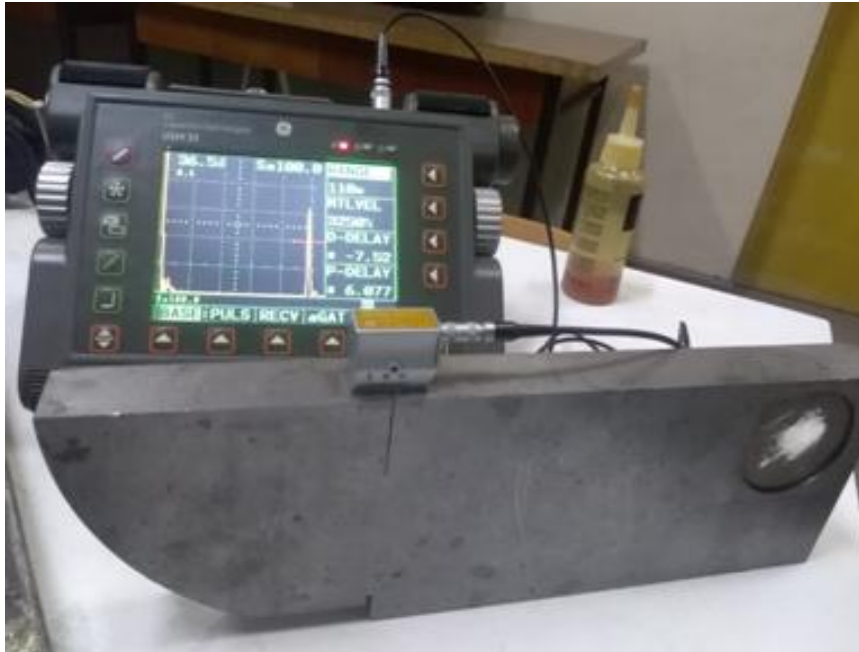
Figure 6 Calibrating the inclined transducer waveguide defectoscope
