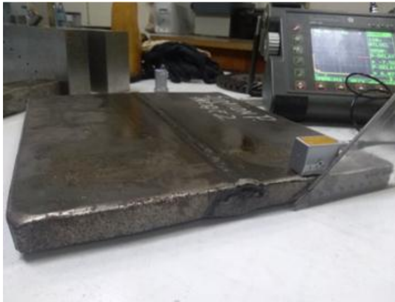
Figure 7 Controlling the specimen itself using an inclined transducer waveguide defectoscope
