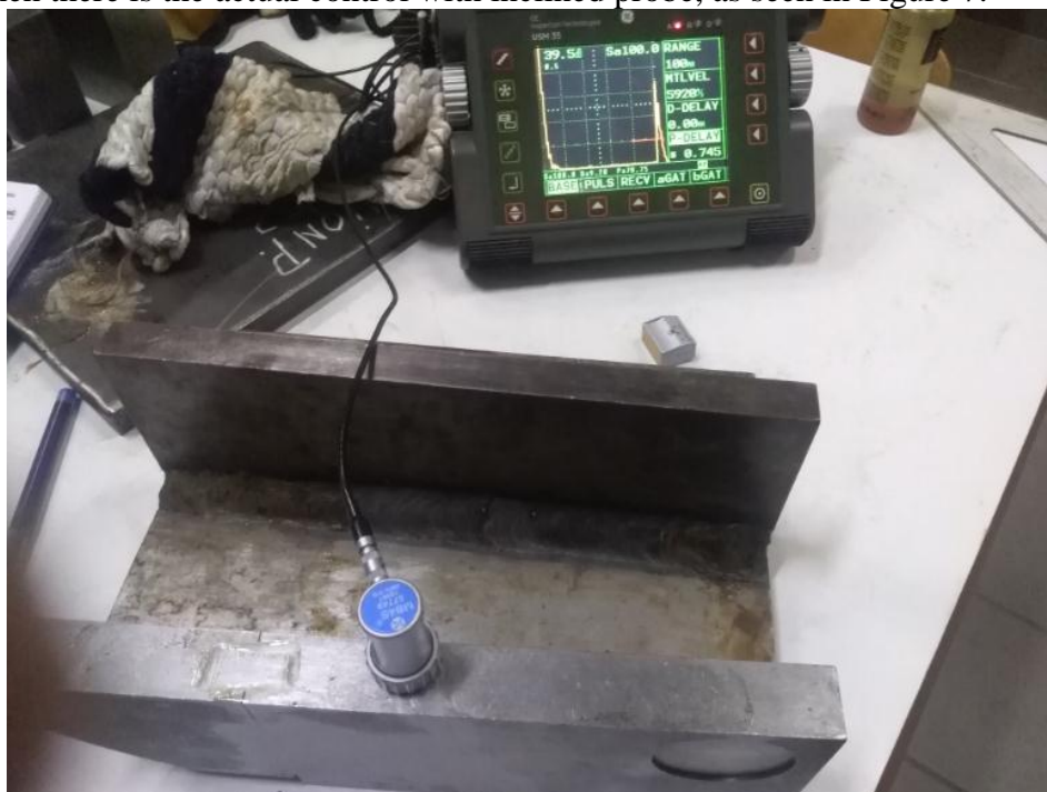
Figure 3 Calibrating the defectoscope with block A1
