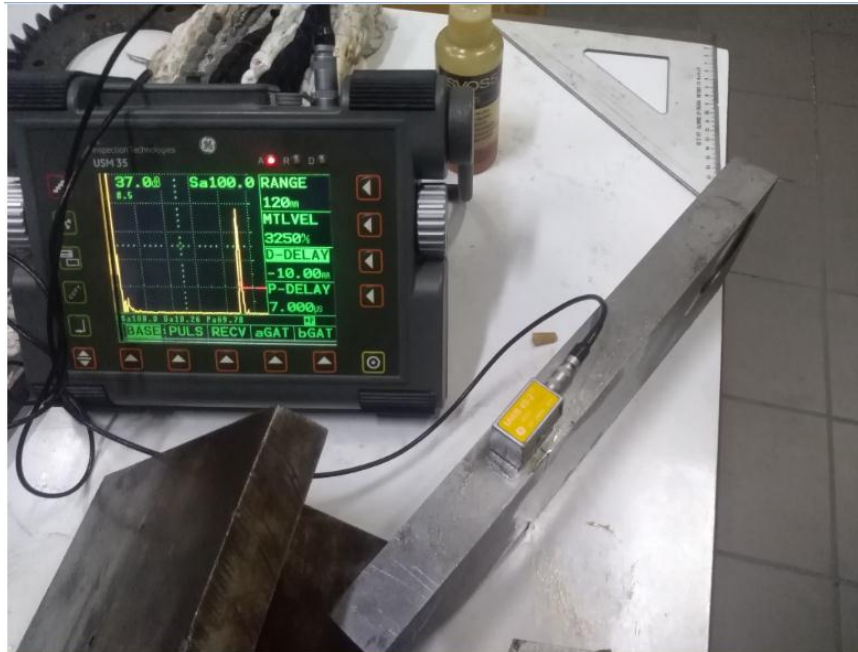
Figure 6 Calibrating the inclined transducer waveguide defectoscope
