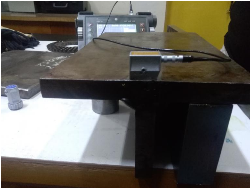
Figure 7 Controlling the specimen itself using an inclined transducer waveguide defectoscope
