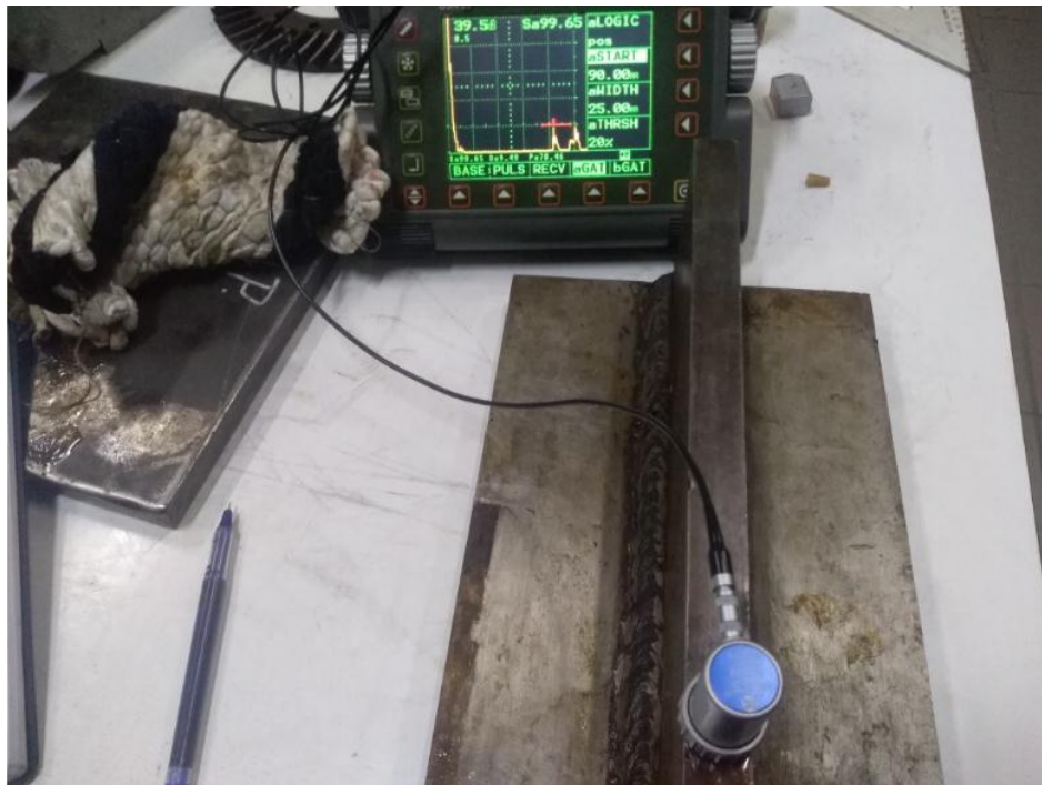
Figure 4 Ultrasonic examination with longitudinal waves on the web of the fillet welded the joint
