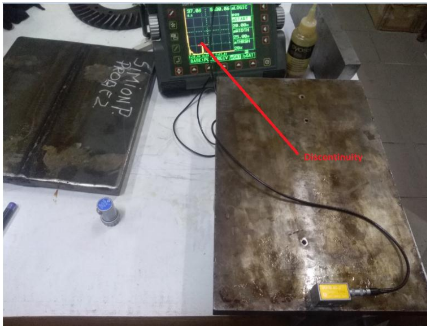
Figure 8 Detection of the discontinuity
