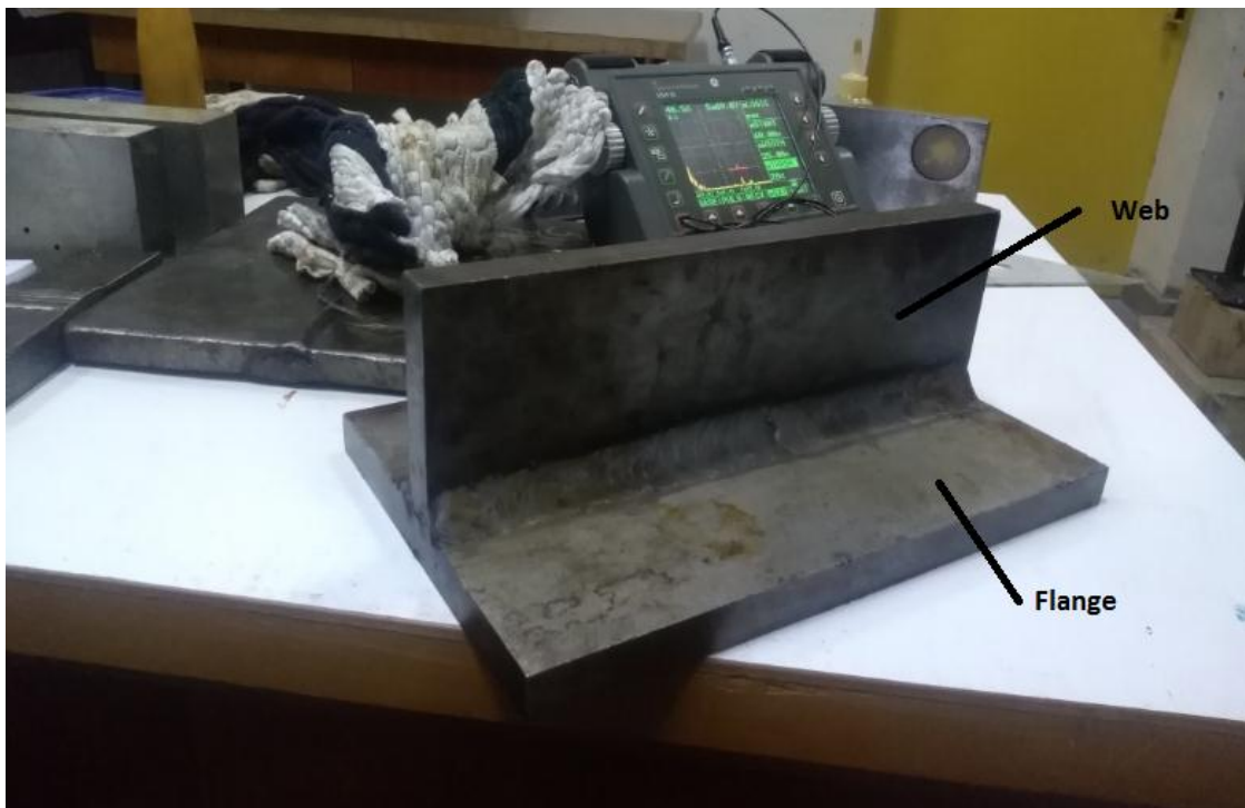
Figure 1 The frillet welded sample subjected to ultrasonic control
