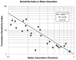
Figure 3: Determination of *n* based on the log-log plot of FRI versus water saturation.
