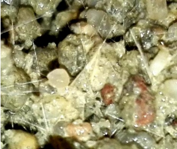
Fig. 2. Uniform dispersion of fibres HP 12 mm at the beginning of mixing.
