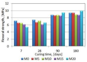
Fig. 8. Flexural strength of mortars with basalt powder addition.
