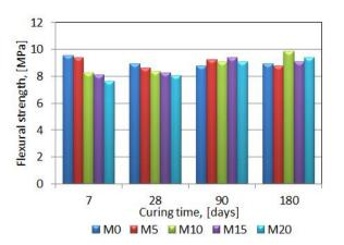
**Fig. 10.** Flexural strength of mortars with ground basalt powder addition.
