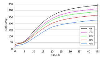
Fig. 6. Cumulative heat release as a function of time and ground basalt powder content.
