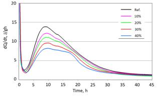
**Fig. 5.** The measured heat flow as a function of time and ground basalt powder content.
