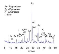
Fig. 2. XRD pattern of the basalt powder.
