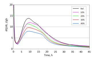
Fig. 3. Measured heat flow as a function of time and basalt powder content.
