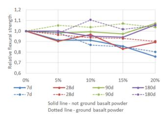
**Fig. 12.** Relative flexural strength of mortars with basalt powder addition.
