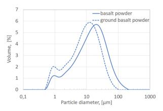
**Fig. 1.** Particle size distribution of basalt powder before and after mechanical activation.
