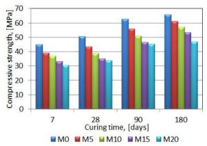
Fig. 7. Compressive strength of mortars with basalt powder addition.
