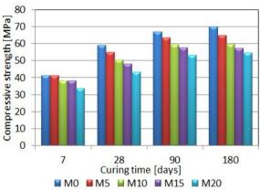
Fig. 9. Compressive strength of mortars with ground basalt powder addition.
