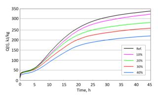
**Fig. 4.** Cumulative heat release as a function of time and basalt powder content.
