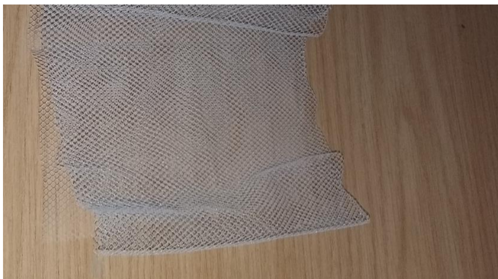
Fig. 4.4: Nylon mesh fabric used for constructing biotrap
