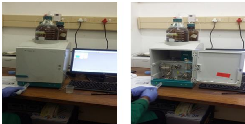
Fig.4.7: IC system used for anion content determination
