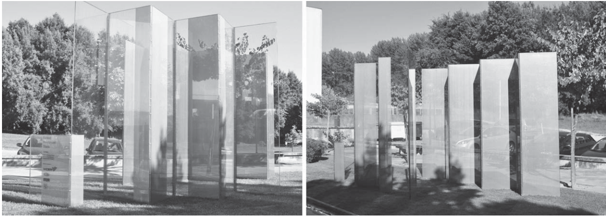
Fig. 16. Different points of view of the finished folded reinforced glass prototype.
