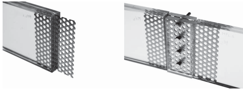
Fig. 1. Concept of extending the reinforcement outwards of the laminate to become the basis for the connection.
