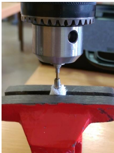
Figure 3. Recording torque value in two implant systems using an electronic torque wrench.
