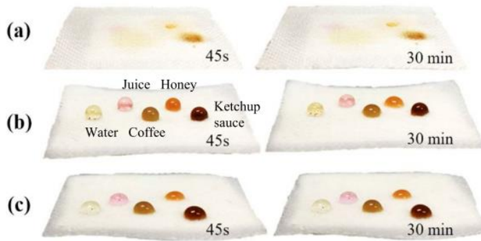
Fig. 11. Optical images of the common household liquid droplets on cotton fabric: (a) uncoated fabric, (b) and (c) before and after 10 cycles of washing of fabric coated with epoxy composite containing 20 vol% SiO 2 -APTES, respectively.
