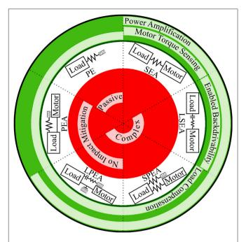
FIGURE 1 | A set of typical implementations of compliance in robotic joints, with main pros and cons shown in green and red respectively.
