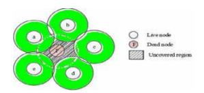
Fuzzy-logic selects one of neighbors of the hole and genetic algorithm determines its destined coordinate in the blank area as demonstrated below.
