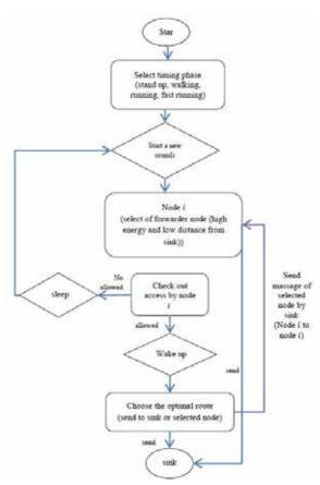
Fig. 3 The flowchart of a node using DTMP protocol
