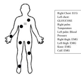
Fig. 1 The location of nodes on the body
