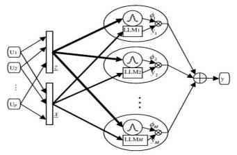
Fig. 1. Topology of a locally linear neuro-fuzzy model (Nelles, 1999)
