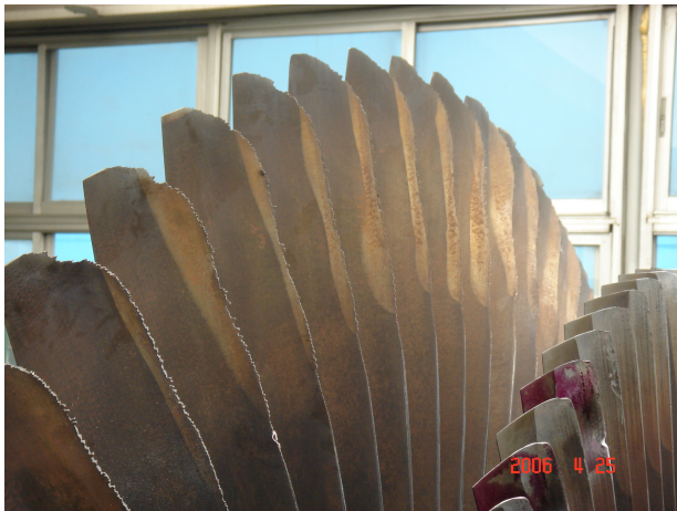
FIGURE 1. Extremely damaged turbine blades.
