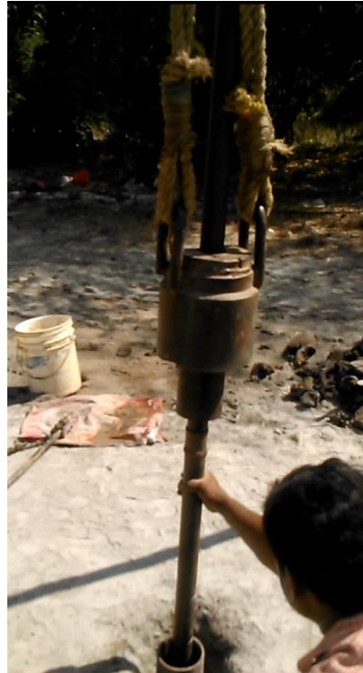
Fig. 2. - Lifting of drop hammer for applying blows
