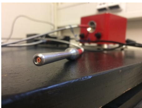
Figure 5 - Probe on the end of fibre optics
