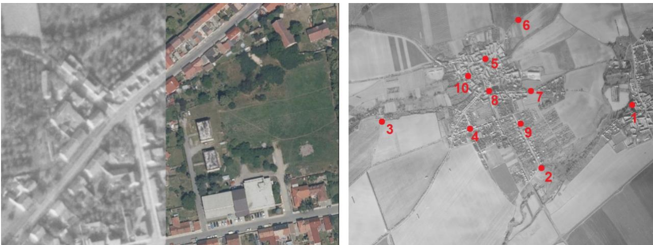
Fig. 6 - Verification of accuracy - visual in urban area (left) and CP distribution (right) Hostouň village – 1969
