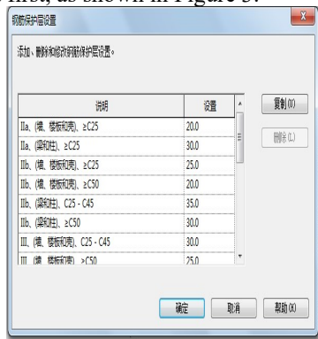
Figure 3. Setting of steel reinforcement protective layer.
