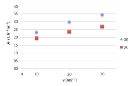
**FIGURE 5.** Effect of the crossflow velocity (v) on the permeate flux  $(J_v)$  for VRF = 10 with the GE and DK membranes at 20 °C and 3 × 10<sup>5</sup> Pa.
