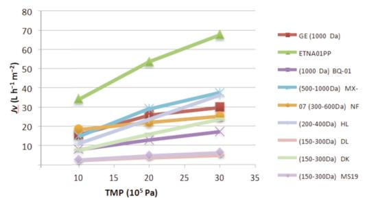
**FIGURE 6.** Effect of the transmembrane pressure (TMP) and molecular weight cut-off (MWCO) on the steady-state permeate flux for experiments performed at  $v = 2 \text{ m.s}^{-1}$  and  $T = 20 \text{ }^{\circ}\text{C}$ .
