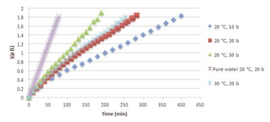
**FIGURE 2.** Evolution of the cumulative permeate volume  $(V_P)$  with processing time for the grape pomace filtration experiments performed with the GE membrane at a tangential velocity  $v = 2 \text{ m.s}^{-1}$ .
