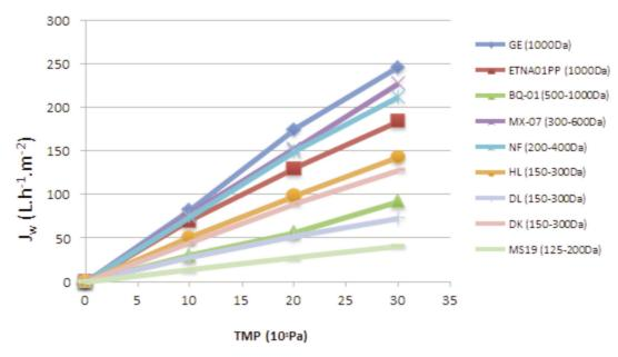
**FIGURE 1.** Hydraulic permeability ( $L_p$ ) for the nanofiltration membranes (T = 20 °C).  $J_w$ , pure water flux; TMP, transmembrane pressure.
