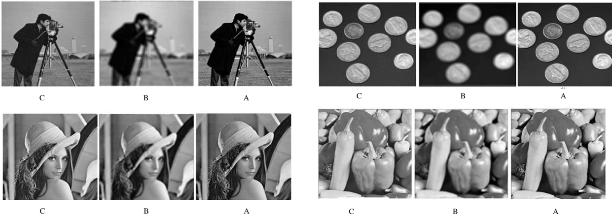
Figure 7. Deblurring results for Cameraman, Coins, Lena, and Peppers: A) Original Image, B) degraded image, and C) restored image by proposed method.
