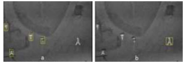
Figure 13. ROIs with possibility of presence of one pedestrian (a) and possibility of presence of several pedestrians (b).
