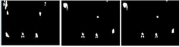
Figure 21. Applying convex hull morphological operator on Fig. 20
