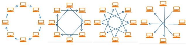
Figure 5. Round method for communication between 8 workers: each worker sends data to another one and receives data from others simultaneously in every iteration.
