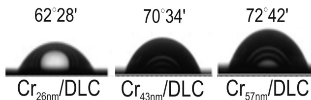
Fig. 6. The contact angles of Cr/DLC thin films with different thickness of Cr layer.
