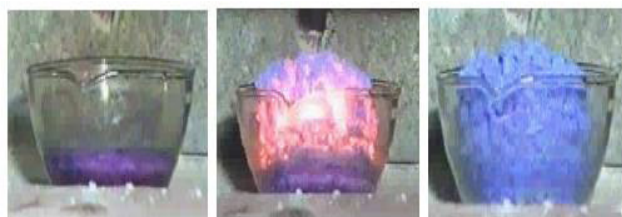
Fig. 1. SCS of mixture on the base of initial batch: 25% \text{Cu}(\text{NO}_3)_2 + 24.6% \text{Ca}(\text{NO}_3)_2 + 50.4% \text{Na}_2\text{SiO}_3 + 3.6% \text{H}_2\text{O} + 40% Urea: initial batch, combustion process and final product.
