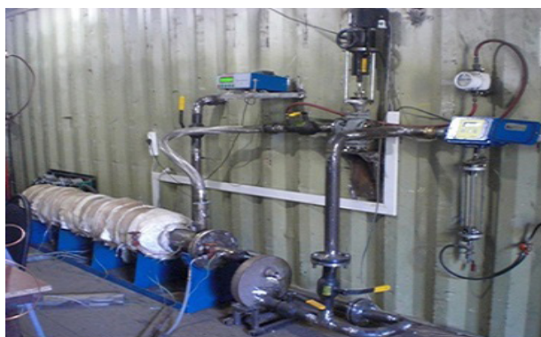
Fig. 9. Reactor part of the pilot unit for the selective oxy-cracking of heavy gas-phase hydrocarbons (a) and results of pilot testing at the conversion of the typical oil associated gas (b) (C 3 H 8 (■), n -C 4 H 10 (▲), n -C 5 H 12 (●), n -C 6 H 14 (◆)). The composition of gas (mol. %): CH 4 – 81.0; C 2 H 6 – 1.22; C 3 H 8 – 17.0; ΣC 4 H 10 – 2.81; ΣC 5 H 12 – 1.50; n -C 6 H 14 – 1.83. The amount of added air – 15%. t_r \sim 1\text{ s} .
