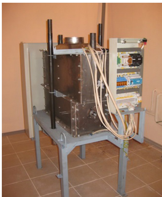
Fig. 6. Pilot matrix converter with natural gas capacity 8 m 3 /h.
