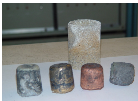
Fig. 4. Bars of metals melted in cylindric glasses: 1 - duraluminium, 2 - bronze, 3 - copper, 4 - cast iron
