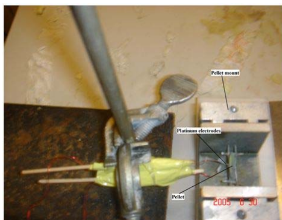
Fig.3. View of experimental setup from above for electric potential measurements. This image was taken before the combustion of the pellets was initiated by a butane torch.
