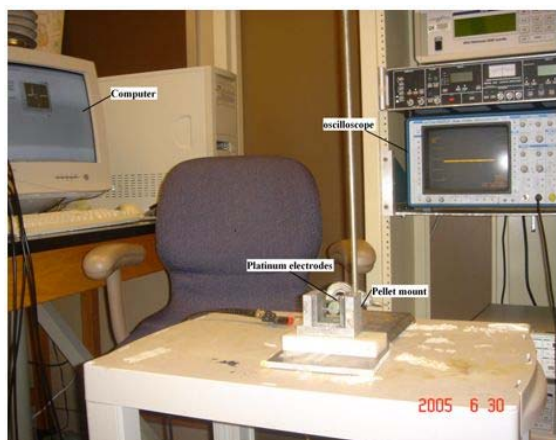
Fig. 2. Front view of experimental setup for electric potential measurements
