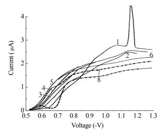
$C_{Te(IV)} = 2.0 \cdot 10^{-4} \text{ M}$  at different concentrations Fe(dipy)<sub>3</sub><sup>2+</sup>: 1 - 0;  $2 - 3.3 \cdot 10^{-5} \text{ M}$ ;  $3 - 6.7 \cdot 10^{-5} \text{ M}$ ;  $4 - 1.3 \cdot 10^{-4} \text{ M}$ ;  $5 - 2.5 \cdot 10^{-4} \text{ M}$ ;  $6 - 5 \cdot 10^{-4} \text{ M}$ ;  $7 - 9.3 \cdot 10^{-4} \text{ M}$ ;  $8 - 1.5 \cdot 10^{-3} \text{ M}$ . Fig. 4. Polarograms for Te (IV) electroreduction in the supporting electrolyte 0.1 M NaF.
