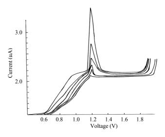
$C_{\text{Te (IV)}} = 2.7 \cdot 10^{-4} \,\text{M}.$   $C_{\text{NaF}}$ :  $1 - 0.005 \,\text{M}$ ;  $2 - 0.01 \,\text{M}$ ;  $3 - 0.05 \,\text{M}$ ;  $4 - 0.1 \,\text{M}$ ;  $5 - 0.2 \,\text{M}$ ;  $6 - 0.5 \,\text{M}$ . Fig. 1. Polarograms for Te (IV) electroreduction in the supporting electrolyte NaF.
