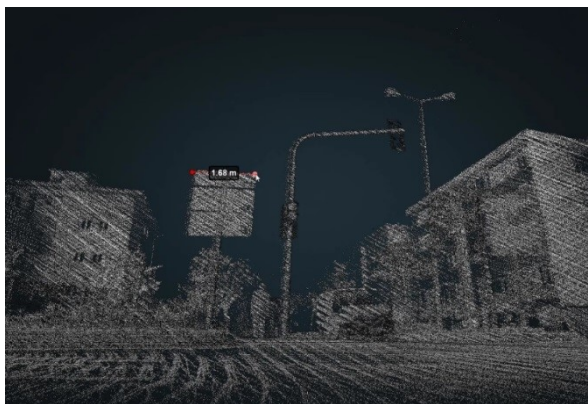
Figure 12: Points cloud of the buildings and other features
