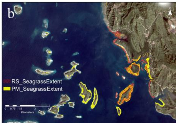
Figure 3. (a) Overlaid patches of mangroves obtained from participatory map (PM, yellow solid) and Sentinel-2 classified image (RS, red hatched); (b) Overlaid patches of seagrass meadows obtained from participatory map (yellow solid) PlanetScope classified image (red hatched).
